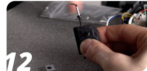
12 With a 2mm hex key, undo the M3x25 Low Profile screw going into the Arrow hotend mount.
