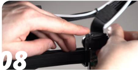
08 Disconnect the toolhead bus cable.
