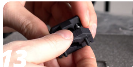
13 Separate the Arrow hotend mount from the Arrow extruder mount.
